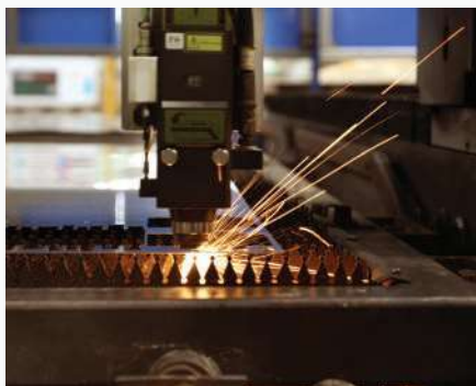
Generates a laser beam that stimulates a lasing material by electrical discharges in a closed container
